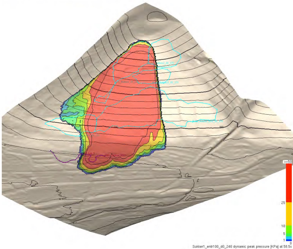
Figure 4.9: Peak pressure in KPa of the Sukkertoppen avalanche with 2,4 m snow depth in the release area and 1 m snow entrainment.
