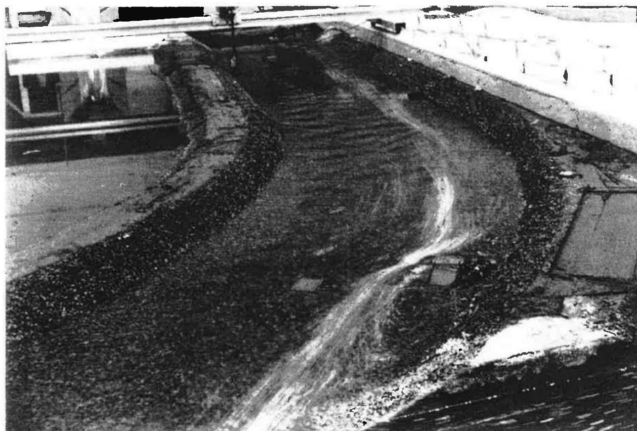
Figur 13. Buner i sving, detaljer strømfordeling. L=32\text{cm} a) 1 bune b) 2 buner S=3,5\text{cm} S/L=10.9
