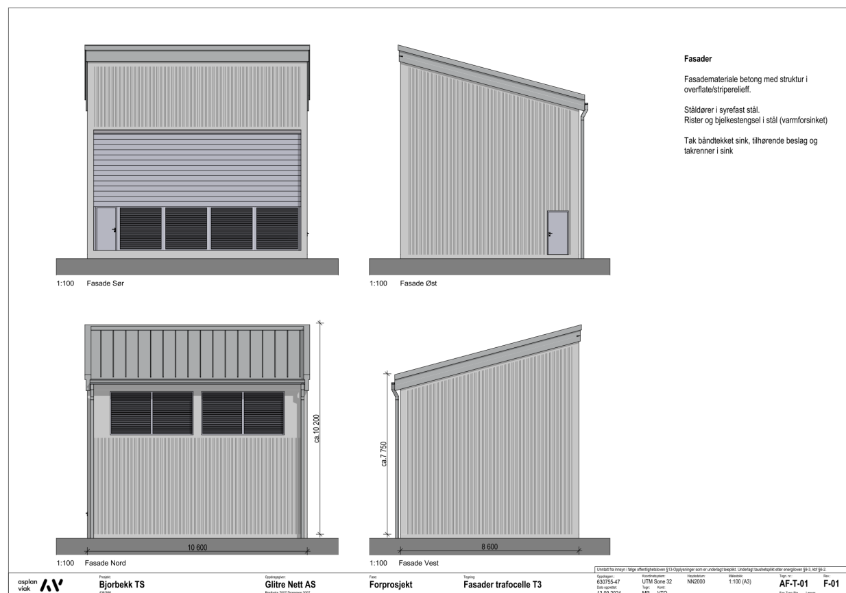
Figur 9: Fasader for ny trafocelle
