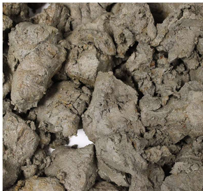
13 – 14m Visuell vurdering: Sandig silt
