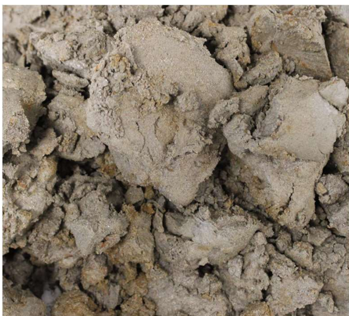
14 – 15m Kornfordeling: Sandig silt
