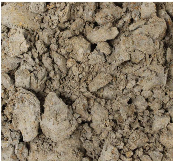
12 – 13m Kornfordeling: Sandig silt
