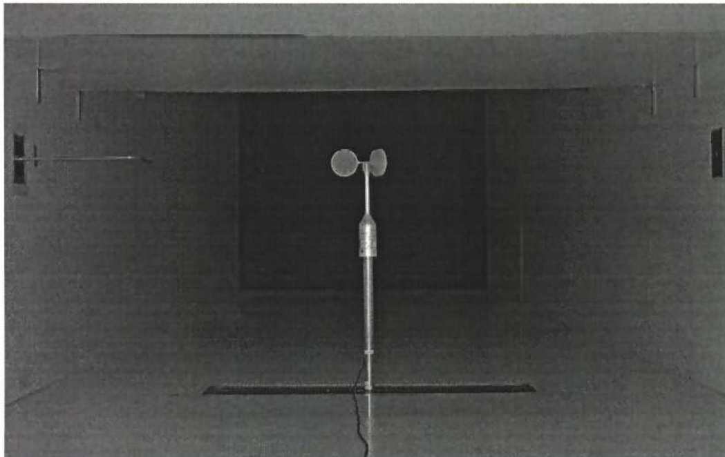
Photo of a cup anemometer in the wind tunnel. The shown anemometer is of the same type as the calibrated one.
