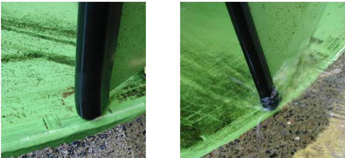
Figure 28. Modified leading edge removing the pinch point.
