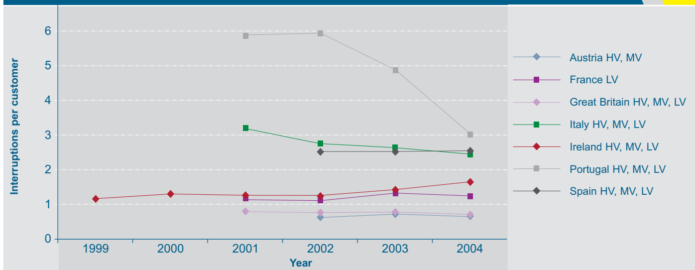
FIG 1.4 UNPLANNED INTERRUPTIONS NOT ATTRIBUTABLE TO EXCEPTIONAL EVENTS Interruptions per customer per year (1999–2004)
