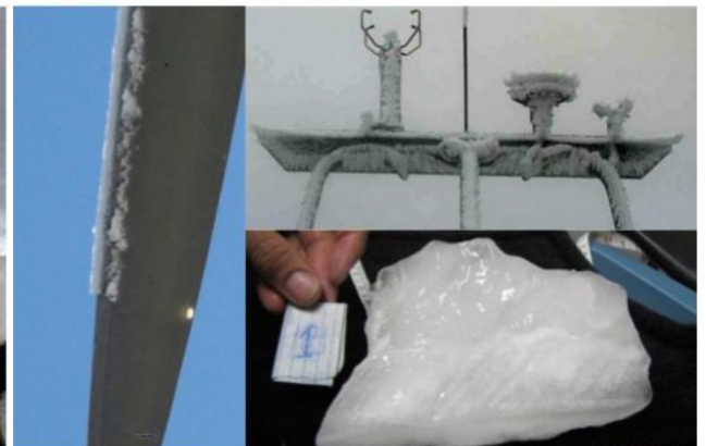
Ice Class Rime 4 (ICR4) – 1.6 to 2.8 kg/m
