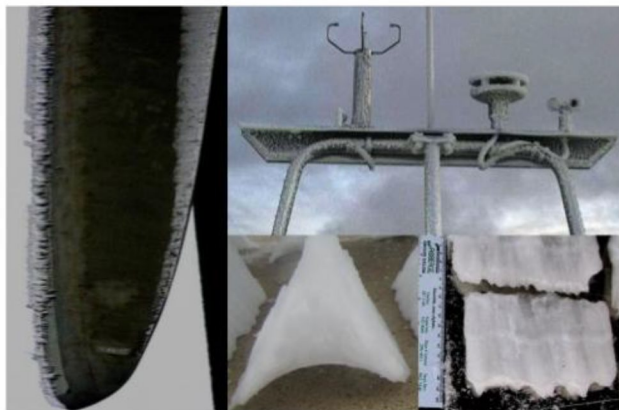
Ice Class Rime 5 (ICR5) – 2.8 to 5.0 kg/m
