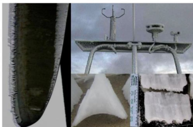
Ice Class Rime 5 (ICR5) – 2.8 to 5.0 kg/m
