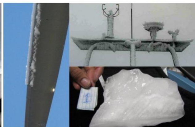
Ice Class Rime 4 (ICR4) – 1.6 to 2.8 kg/m
