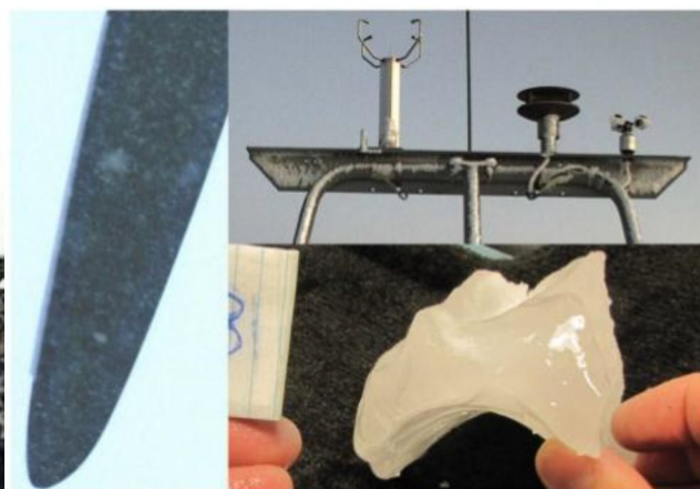
Ice Class Rime 4 (ICR4) – 1.6 to 2.8 kg/m
