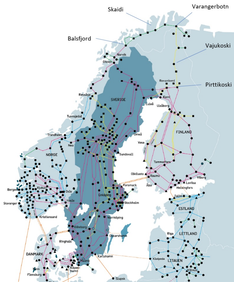
Figure 1 The transmission grid in the Nordic and Baltic countries, where the key points for this project have been pointed out by DNV GL. (Svenska Kraftnät, 2013)
