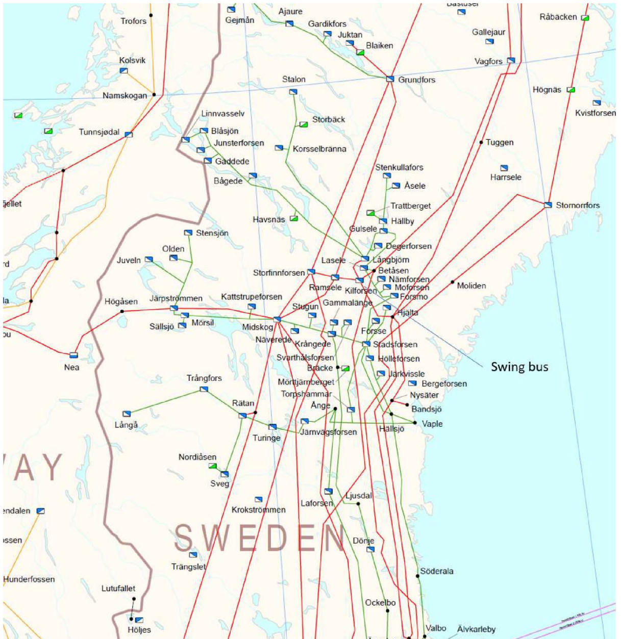
Figure 9: The geographical location of the swing bus, closely connected to the 4 transmission lines between SE1 and SE2.
