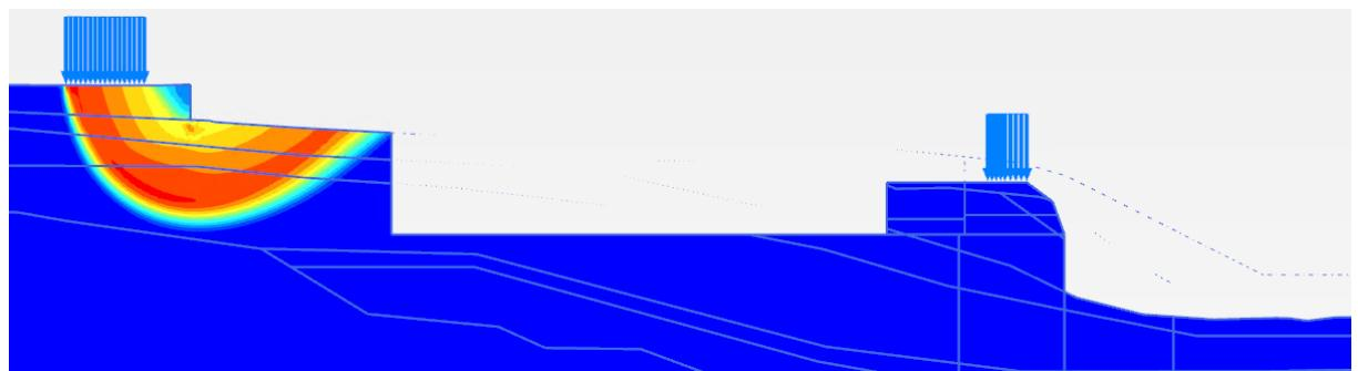
Figur 40: Snitt R5 - ADP, Beregning 4-1, bruddmønster
