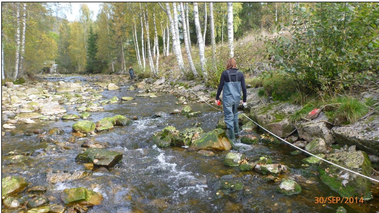
Figure 23: measuring the transects on station 3 at low water velocity. Seen in upstream direction. Photo: © Jan Heggenes.
