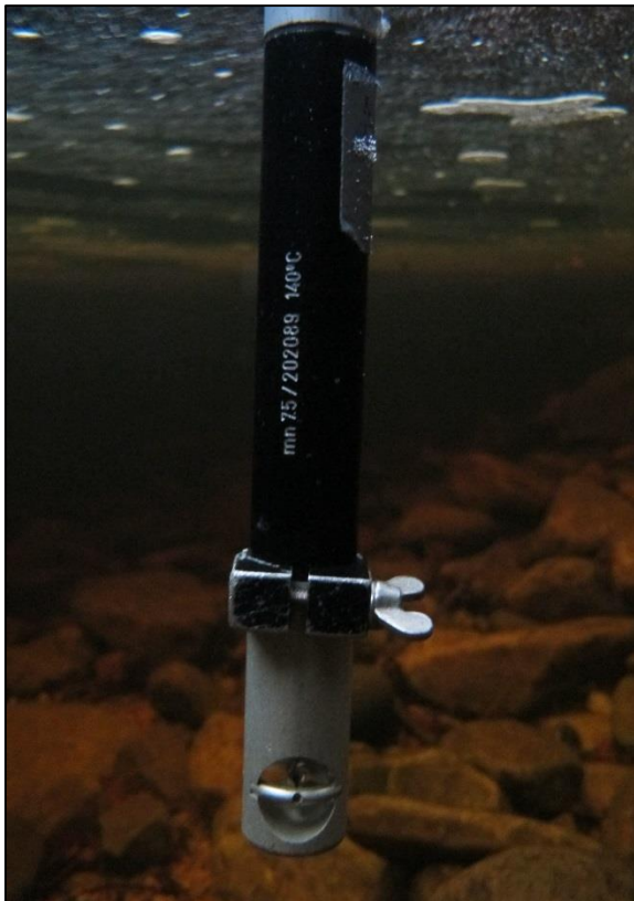
Figure 7: measures of water velocity taken with a portable mechanical flowmeter. Photo: © Tobias Andrés.
